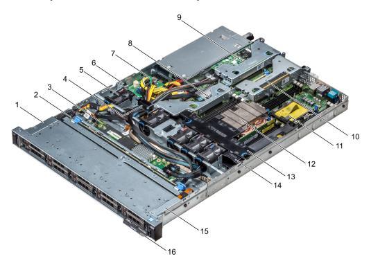
Note The graphic above shows a configuration of ten internal drives installed in the front drive cage of the appliance; however, only a four drive configuration installed in the front drive cage is available with LiveCapture 1100.
