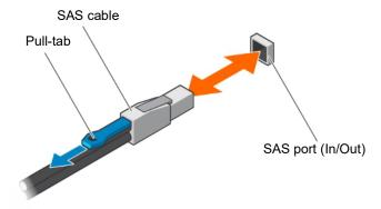
**Note** It may be necessary to remove the handle on the rear of the appliance in order to connect the SAS external cascading cable into the left RAID port of the RAID controller.
